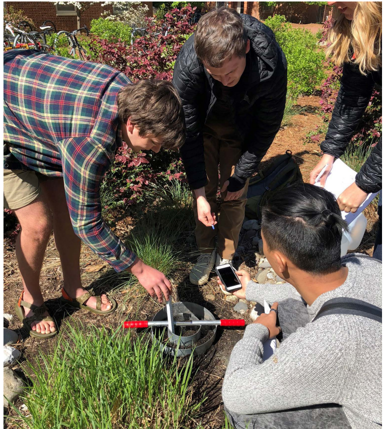
Figure 8. Double-ring Infiltrimeter Field Demonstration (Credit: Emily McCoy)
