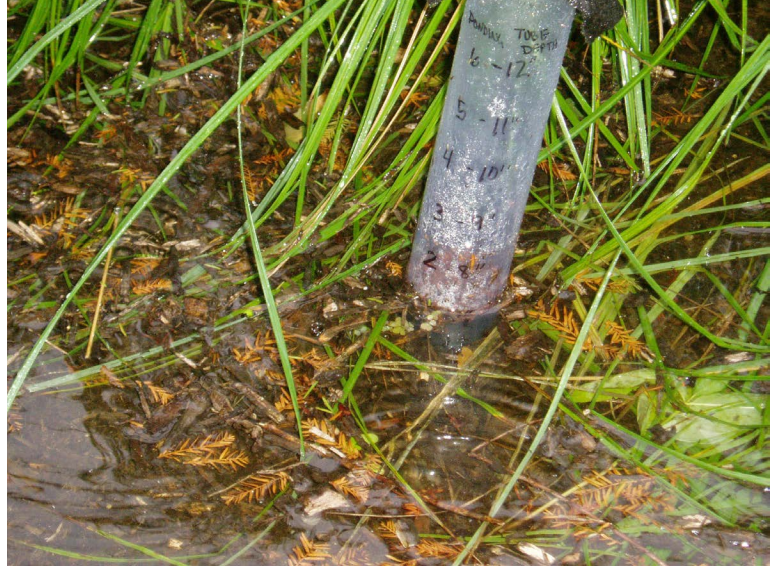
Figure 14. DIY Water Depth Gauge (Credit: Emily McCoy)
