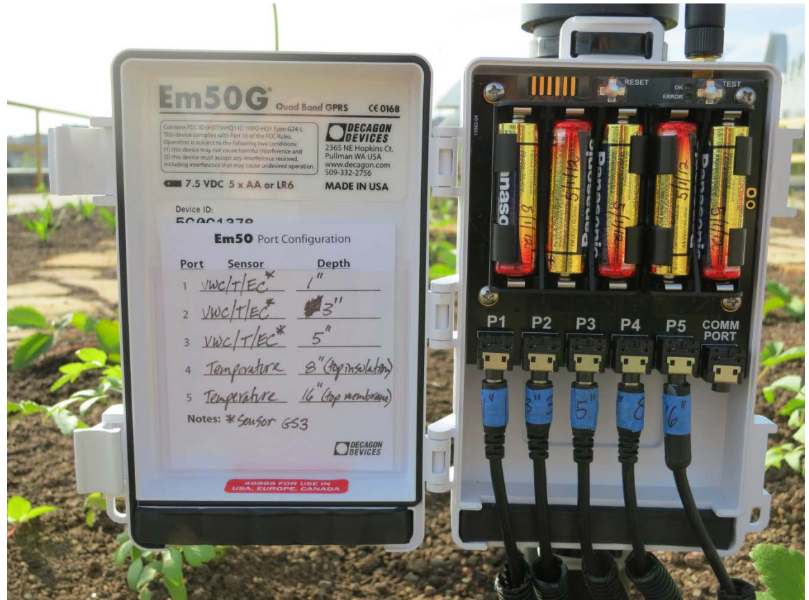
Figure 11. Data Logger (Credit: John Buck, CPSS Civil & Environmental Consultants, Inc., Pittsburgh, PA)
