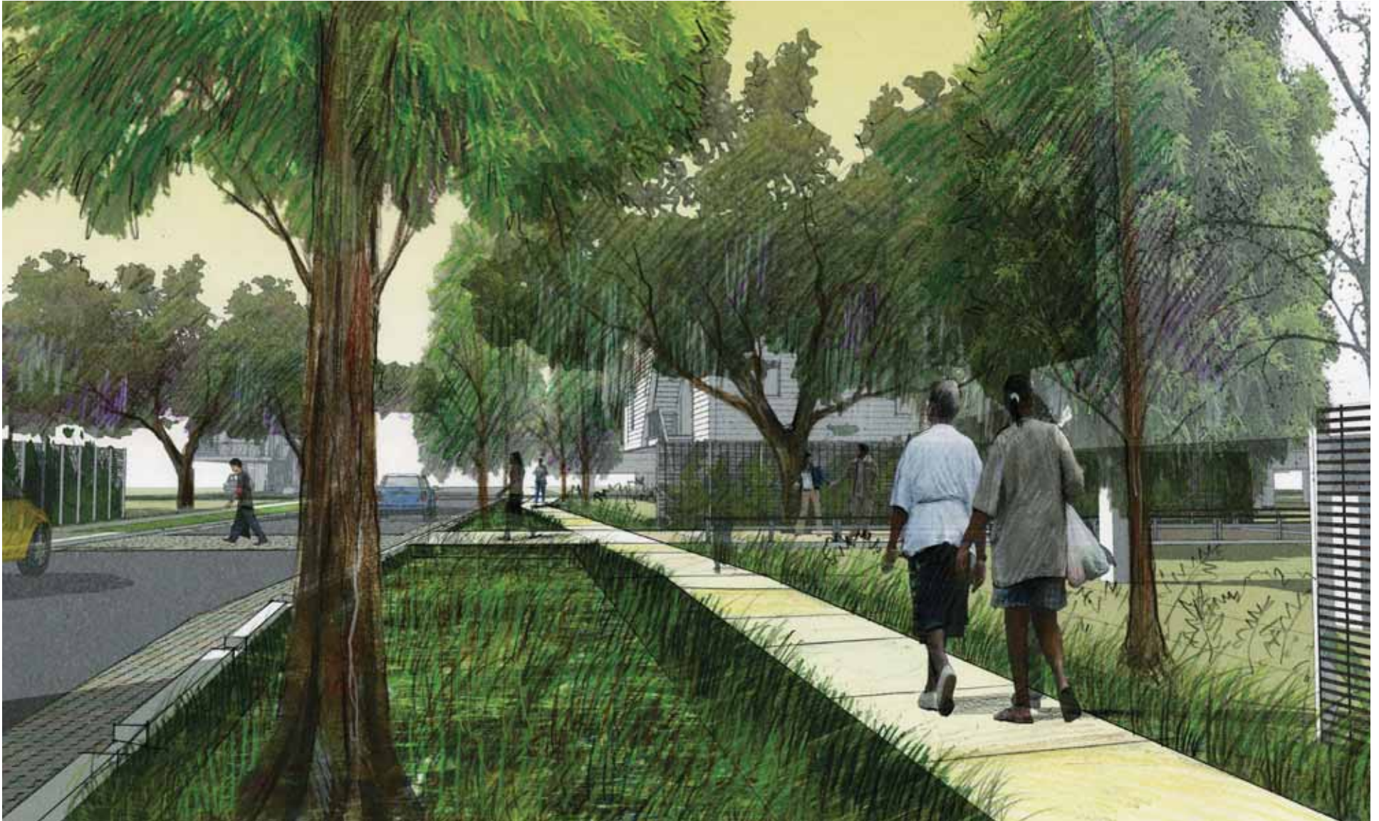
Illustration showing post-construction sustainable stormwater and traffic-calming strategies along North Derbigny Street in the Lower Ninth Ward (Image created by Siteworks Studio for the L9SIP project).
